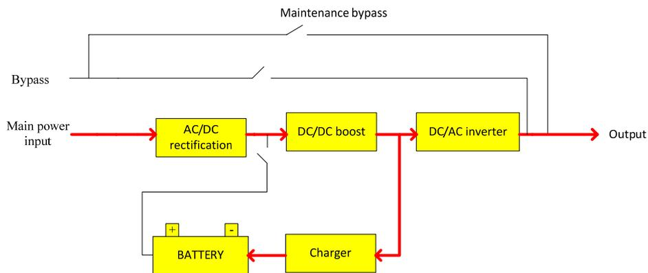
Figure 1.4 Working Process Chart under Main Power Mode
