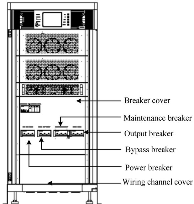
Figure 2.8 Front View of 40-60KVA
