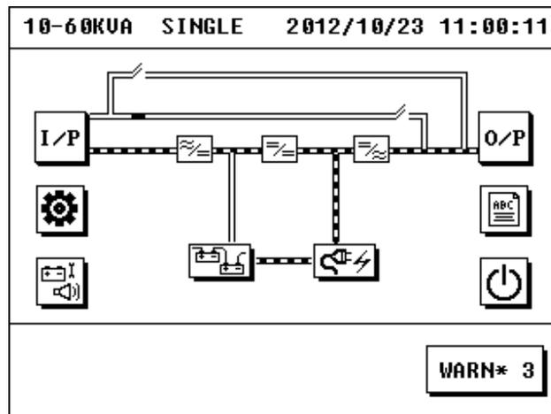
Figure 3.6 Operations under Main Power
