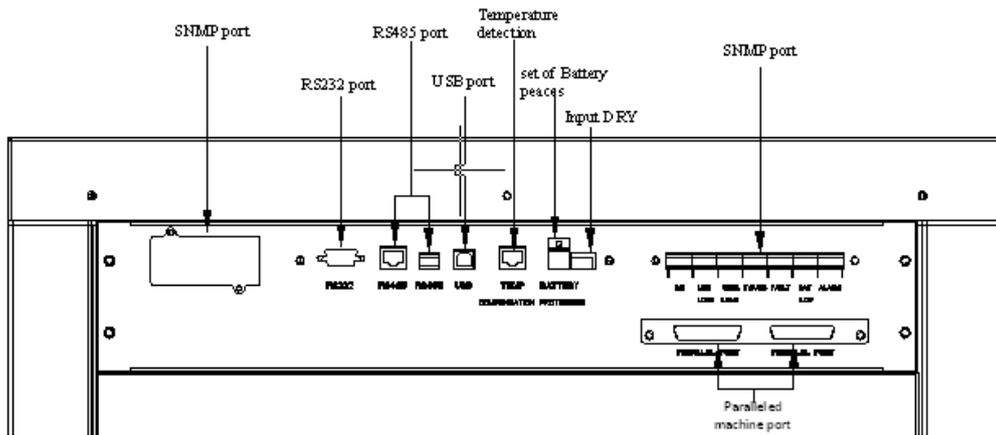
Figure 1 Chart of 10-120KVA Communication Port
