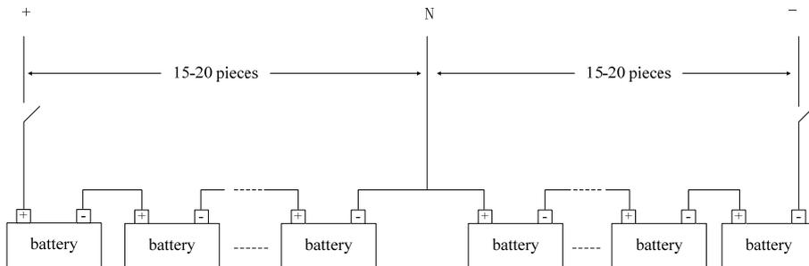
Figure 2.13 Battery Connection Chart
