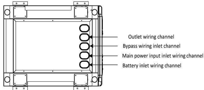
Figure 2.5 Inlet and Outlet Wiring Channel of 10-60K
