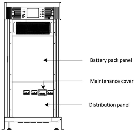
Figure 2.7 Front View of 10-30KVA
