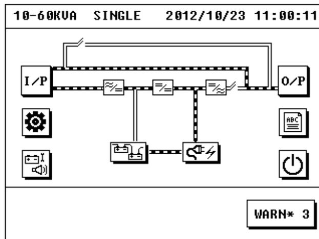
Figure 3.13 Bypass Mode
