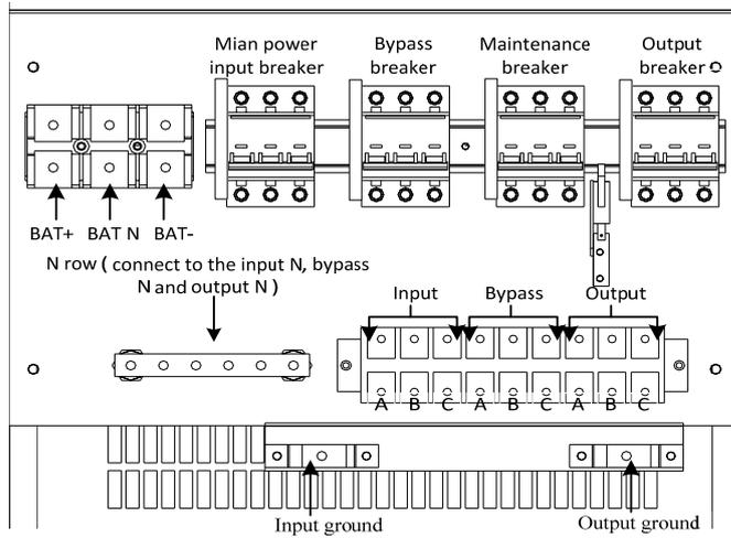
Figure 2.10 Distribution Wiring Diagram of 10-30KVA series
