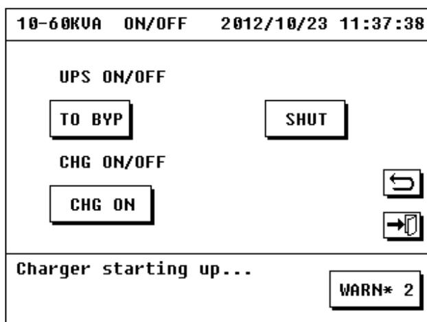
Figure 3.15 On/Off Interface of Charger
