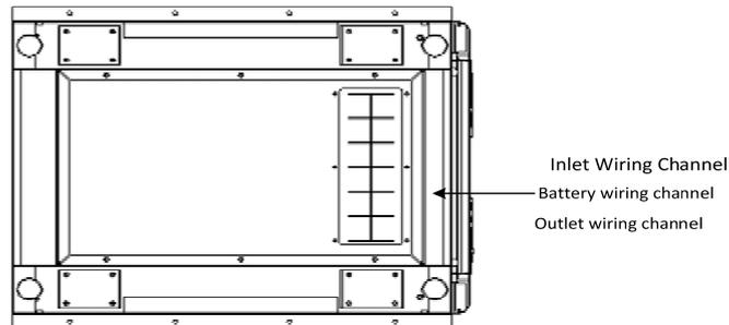
Figure 2.6 Inlet and Outlet Wiring Channel of 80-120K
