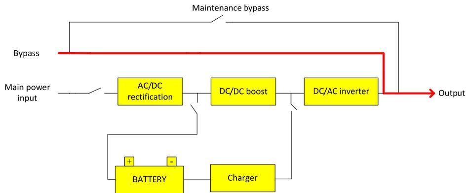
Figure 1.6 Working Process Chart under Bypass Mode
