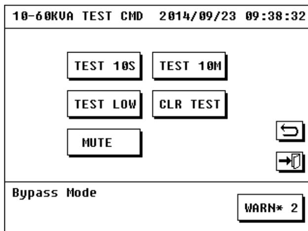
Figure 3.46 Interface of Self-test and Mute off
