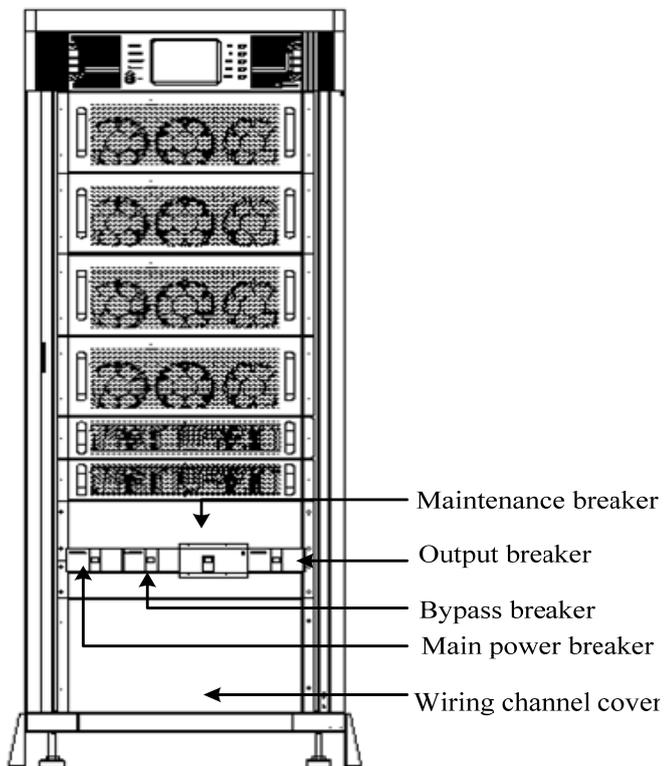
Figure 2.9 Front View of 80-120KVA
