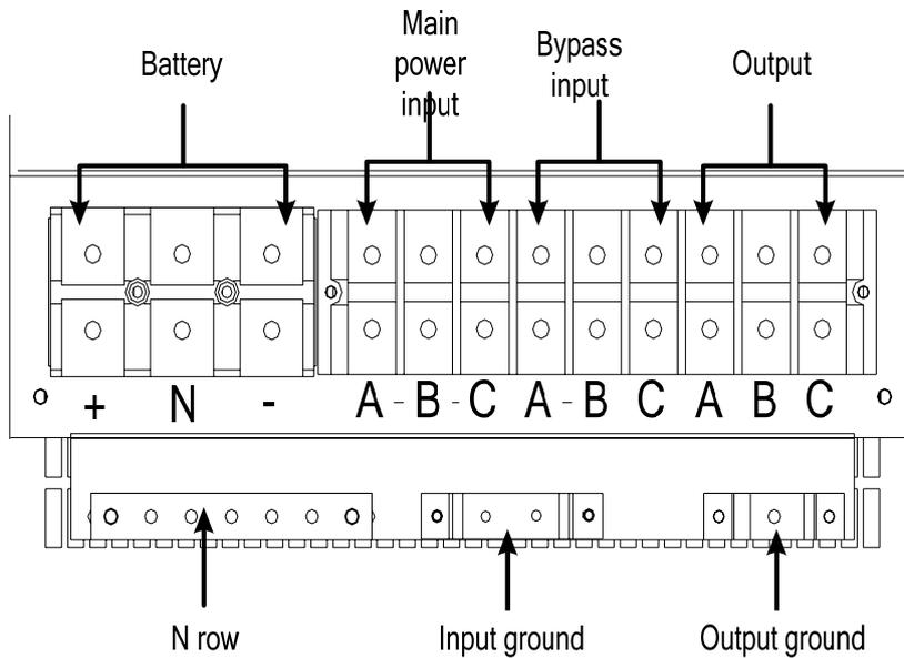
Figure 2.11 Distribution Wiring Diagram of 40-60KVA series
