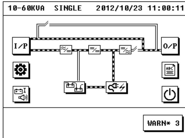
Figure 3.19 Bypass Mode
