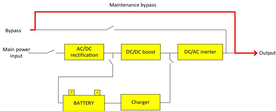
Figure 1.7 Working Process Chart under Maintenance Bypass Mode
