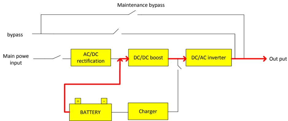
Figure 1.5 Working Process Chart under Battery Mode
