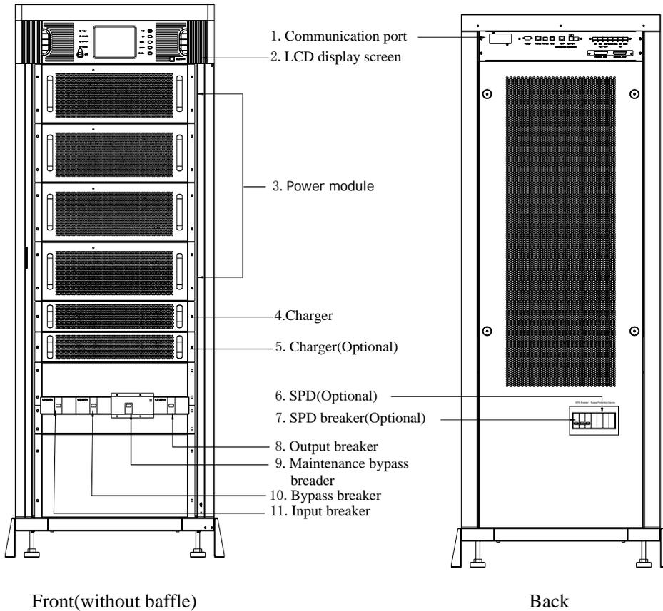
Figure 1.3 Structure of 80-120KVA series
