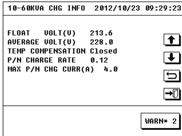
Figure 3.24 Interface of Charger Parameter
