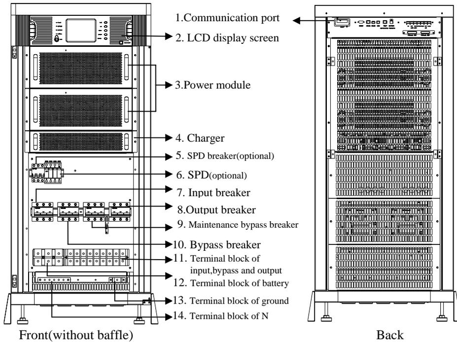
Figure 1.2 Structure of 40-60KVA series
