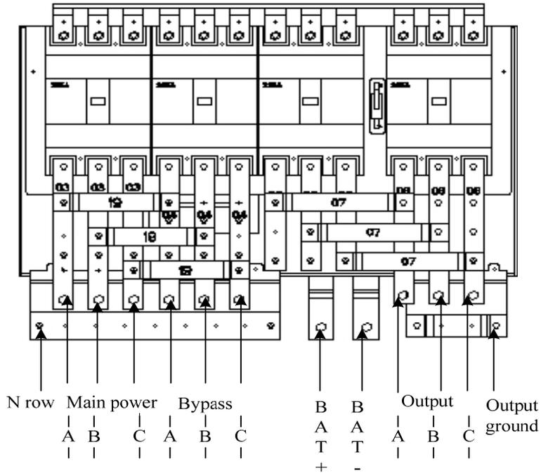
Figure 2.12 Distribution Wiring Diagram of 80-120KVA series
