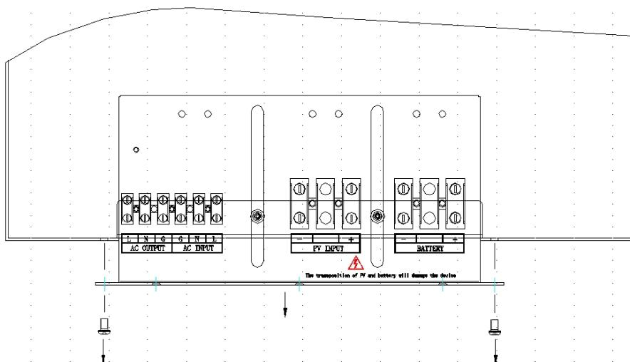
2) According to the identification and connect the cables
