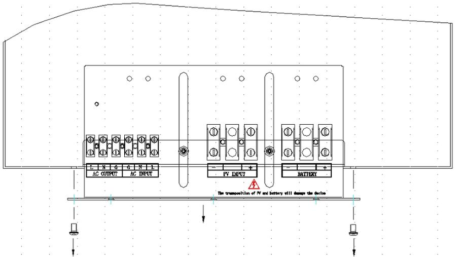
2) According to the identification and connect the cables
