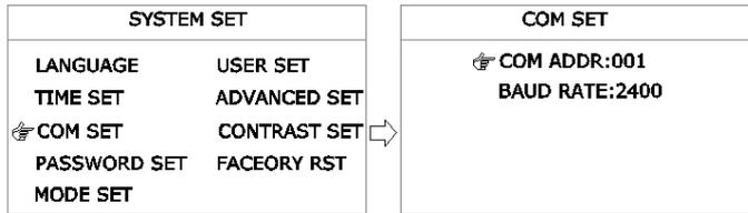
Wrong settings will lead to the inverter communication abnormal, must be set by the professional person, the highest communication baud rate shall below 9600bps.
